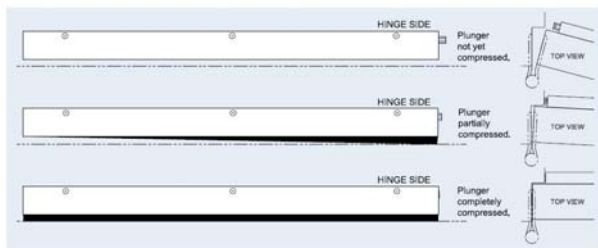
Functioning of an automatic door bottom
